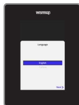
Re-attach the display until a "click" is heard. You can now restore power to the circuit and power up the thermostat. Follow the on screen instructions to set up your system. Once set up a QR Code will appear.
